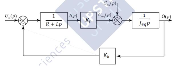
$$\Omega_{m}(p) = \frac{\frac{K_{i}}{(R+Lp)J_{eq}p}}{1 + \frac{K_{i}K_{b}}{(R+Lp)J_{eq}p}} U_{m}(p) + \frac{\frac{1}{J_{eq}p}}{1 + \frac{K_{i}K_{b}}{(R+Lp)J_{eq}p}} C_{Req}(p)$$
